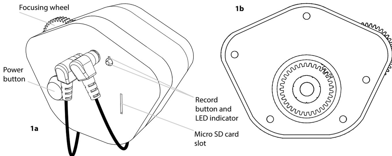
**1a** The RTEK camera module has the capability to capture video simply at the push of a button. Before turning on the camera module, place the micro SD card into the slot on the back of the camera module.
