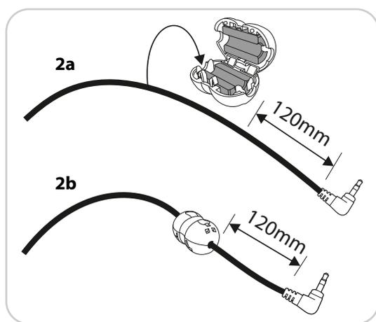
**2a** Place the LCD screen & illuminator module cable into the ferrite approximately 120mm from the end of the right-angle plug.
