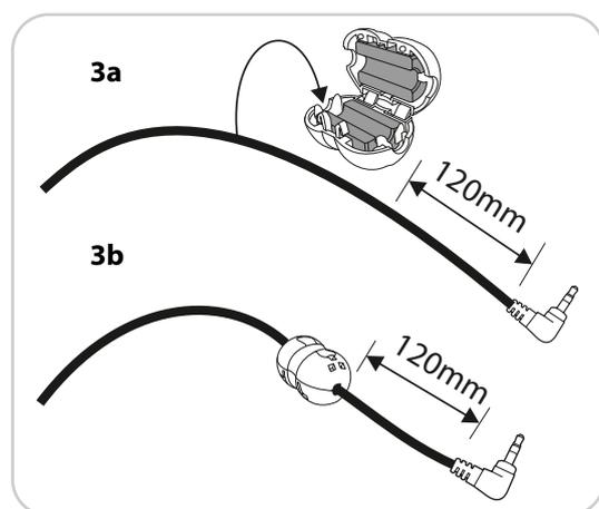
**3a** Place the LCD screen & illuminator module cable into the ferrite approximately 120mm from the end of the right-angle plug.
