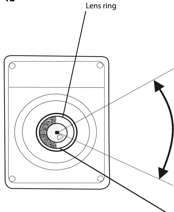
The camera module will require adjustment prior to use. This will guarantee that the scope reticle is in focus when viewed on the LCD screen. The focal distance is factory set, this will usually allow focus to be achieved within a couple of turns of the abrasive ring anti-clockwise.
